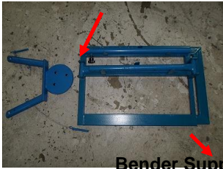
Bender Support Base Image of support base parts
